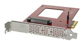
Get ultra-fast data access by adding an NVMe U.2 SSD to your computer. This U.2 to PCIe adapter lets you add a high-speed, U.2 (4-lane PCIe) 2.5" NVMe SSD, such as the Intel 750 Series drive, to a PC with an available x4 PCI Express expansion slot.
